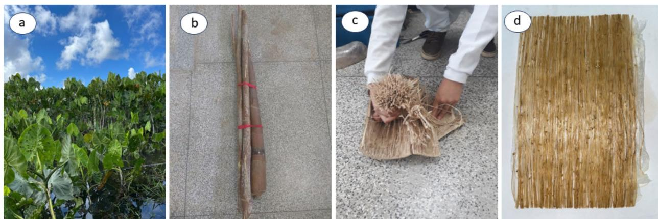
**Fig. 1.** Aninga fiber extraction: (a) Aninga plant; (b) Stem on maceration process; (c) Fiber manual extraction; (d) Unidirectional sheet.
