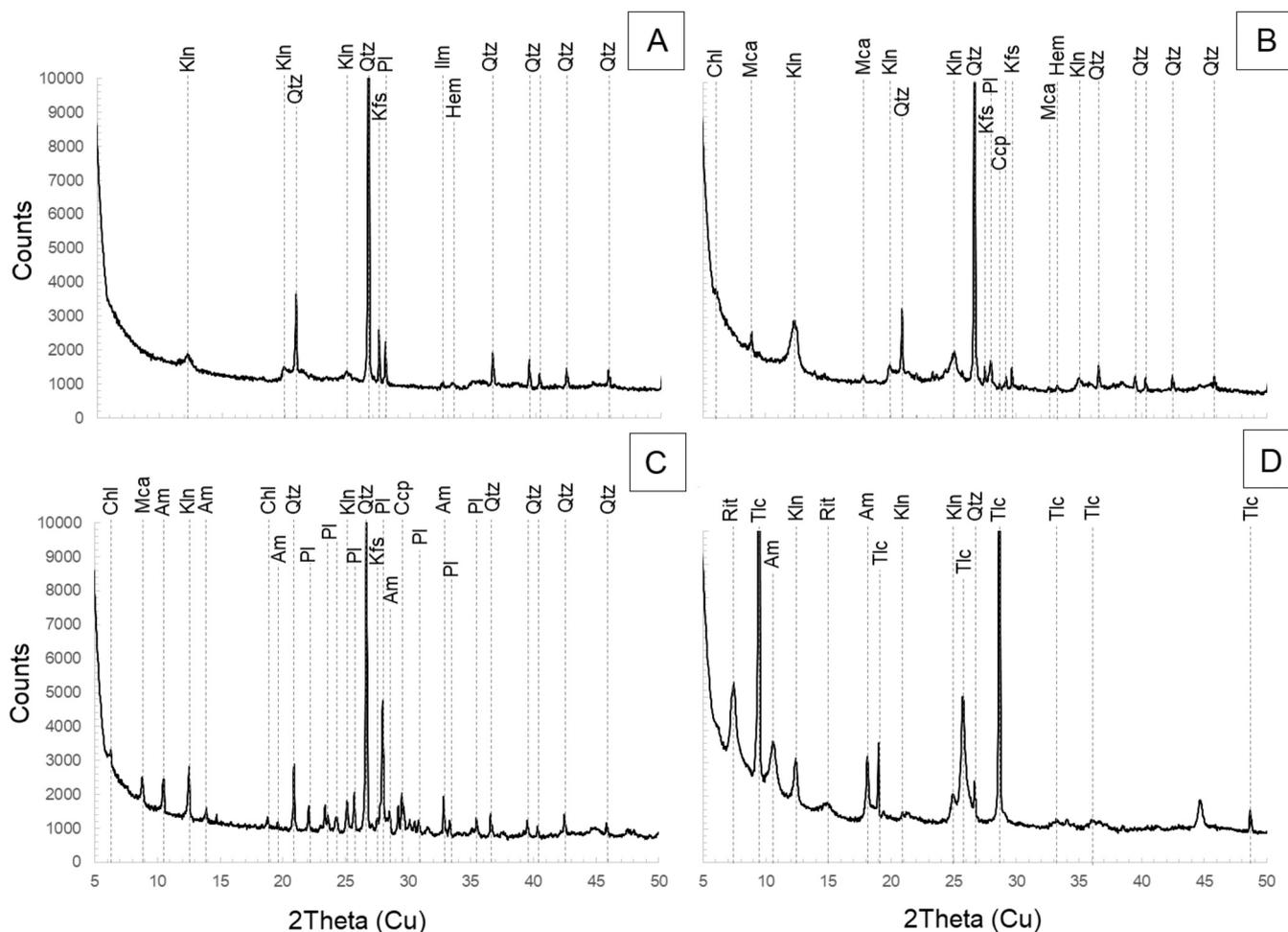
**Fig. 2.** X-ray diffractograms of samples from forest soil (A), artisanal overburden (B), industrial tailings (C), and artisanal rock waste (D) collected in copper mining areas in the eastern Amazon - Brazil. Qtz - Quartz, Hem - Hematite, Mca - Mica, Kln - Kaolinite, Kfs - K-Feldspar, Pl - Plagioclase, Chl - Chlorite, Am - Amphibole, Ilm - Ilmenite, Ccp - Chalcopyrite, Rit - Richterite, Tlc - Talc.
