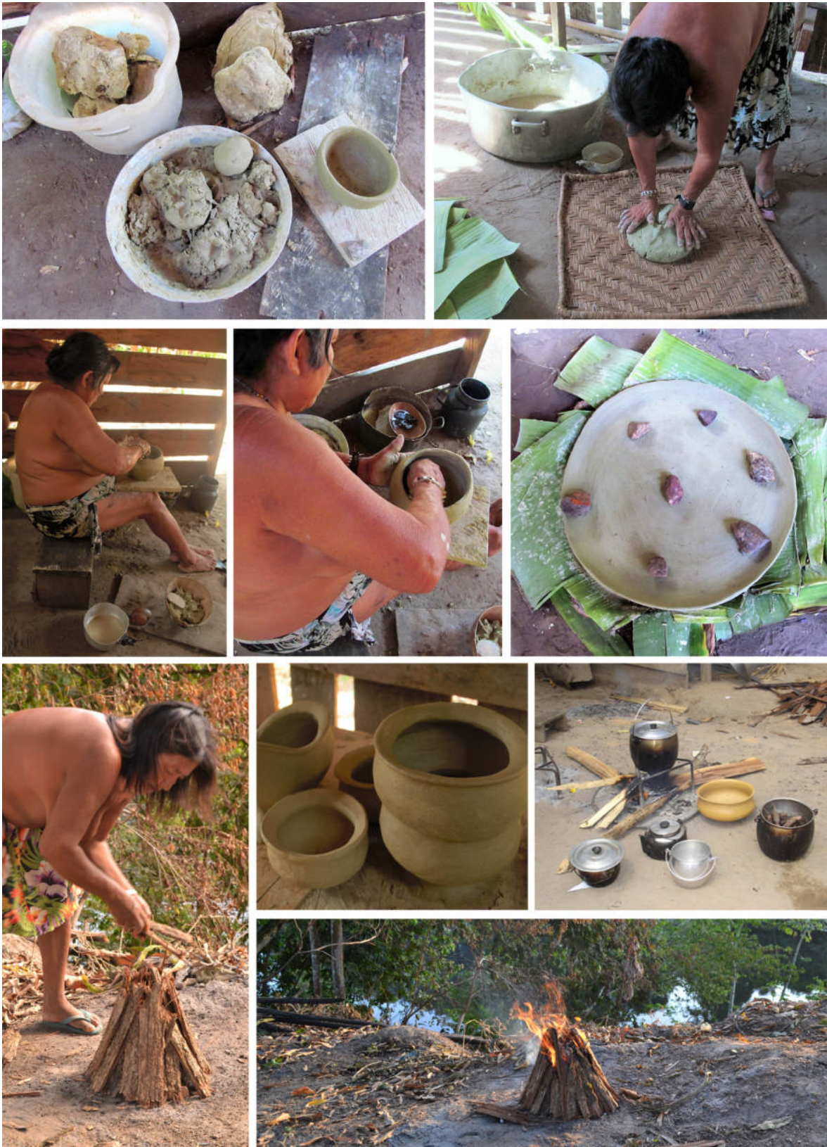
Plate 1. Steps in the making of Wayana ceramics. a) Raw materials. b) Making a griddle. c) Making a pot. d) Smoothing out the internal surface. e) Drying the griddle. f) Drying the pot. g) Drying next to the fire. h) Preparing the fire. i) Firing the ceramics.
